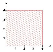
2. Divide x into two regions and y into two regions. This cuts the domain into four rectangles with length  $\Delta x = 2$  and width  $\Delta y = 2$ .
