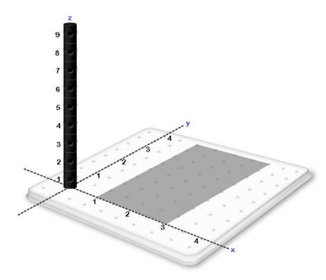
The second datum from the integral is  $\int_0^x$  ... dy indicating that for every value of x between x = 1 and x = 3, we will accept values of y that reside between y = 0 and y = x.
